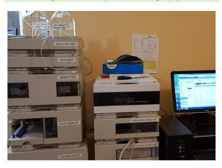
High Pressure Liquid Chromatography (HPLC) is a powerful tool to determine the components in a food. It can be applied to many different types of nutrients: proteins, carbohydrates, phytochemicals, vitamins and other bioactives. HPLC is used for "profiling", for example to make sure a food has the right balance of active constituents. It is especially powerful when you want to know how much of an active ingredient is in your product or how pure it is (quantitative analysis).
